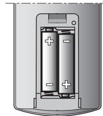
When inserting new batteries, make sure the positive / negative terminals are connected correctly.
