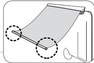
**EN** Pull the legs completely out, and, lower them together to the ground simply by turning on pins and without forcing.
