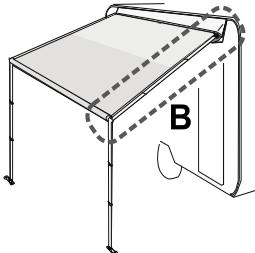
**EN** Tighten the rafter until the fabric is sufficiently taut.
